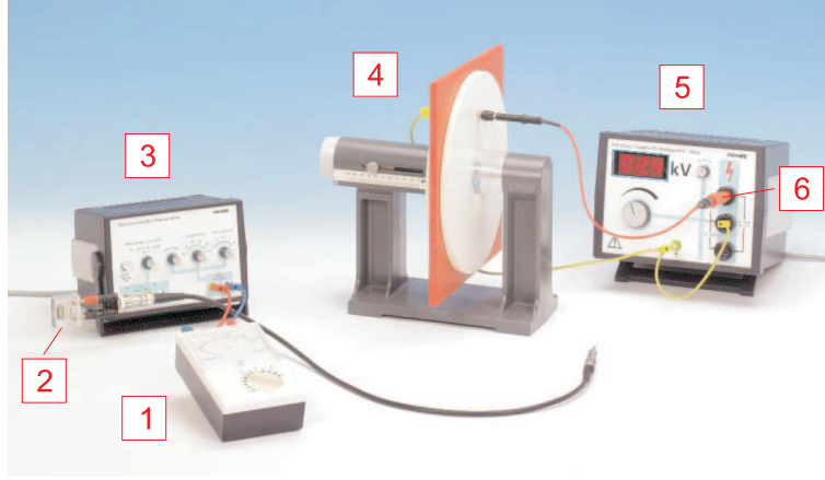
Figure 1.1: Experimental set-up: [1] – voltmeter, [2] – reference capacitor, [3] – universal measuring amplifier, [4] – measuring plate capacitor (with inserted dielectric sample), [5] – high voltage power supply, [6] – high-value protective resistor.
